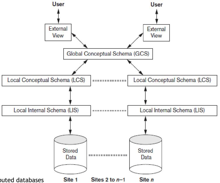
Figure 3 Schema architecture of distributed databases
